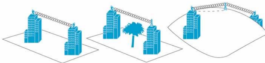
Figure 2. Crossing Great Distances with Cisco Aironet Bridge Antennas
